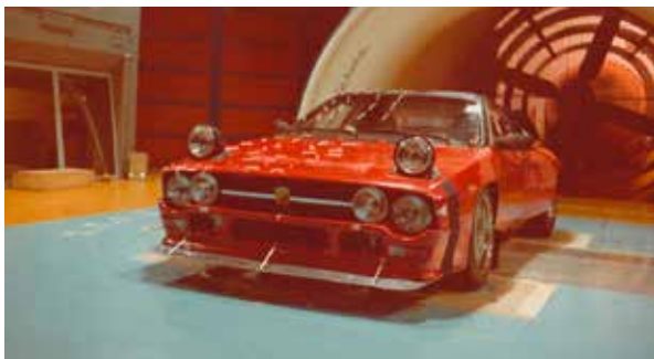
Chassis SE037-001 in the Pininfarina wind tunnel
